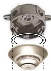
Detector mounts on a standard 4-inch octagon box or 4-inch exterior cast metal back box and gasket) as shown here.
