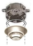
The detector is installed using rain-tight conduit and a standard, approved weatherproof electrical enclosure as shown above. A neoprene (or similar gasket supplied with the back box), is installed between the detector's seal plate and the back box. The wire leads are connected to the initiating circuit inside the enclosure. Unused threaded openings are sealed with threaded plugs. A decorative anodized aluminum cover ring snaps over the detector to complete the installation.
